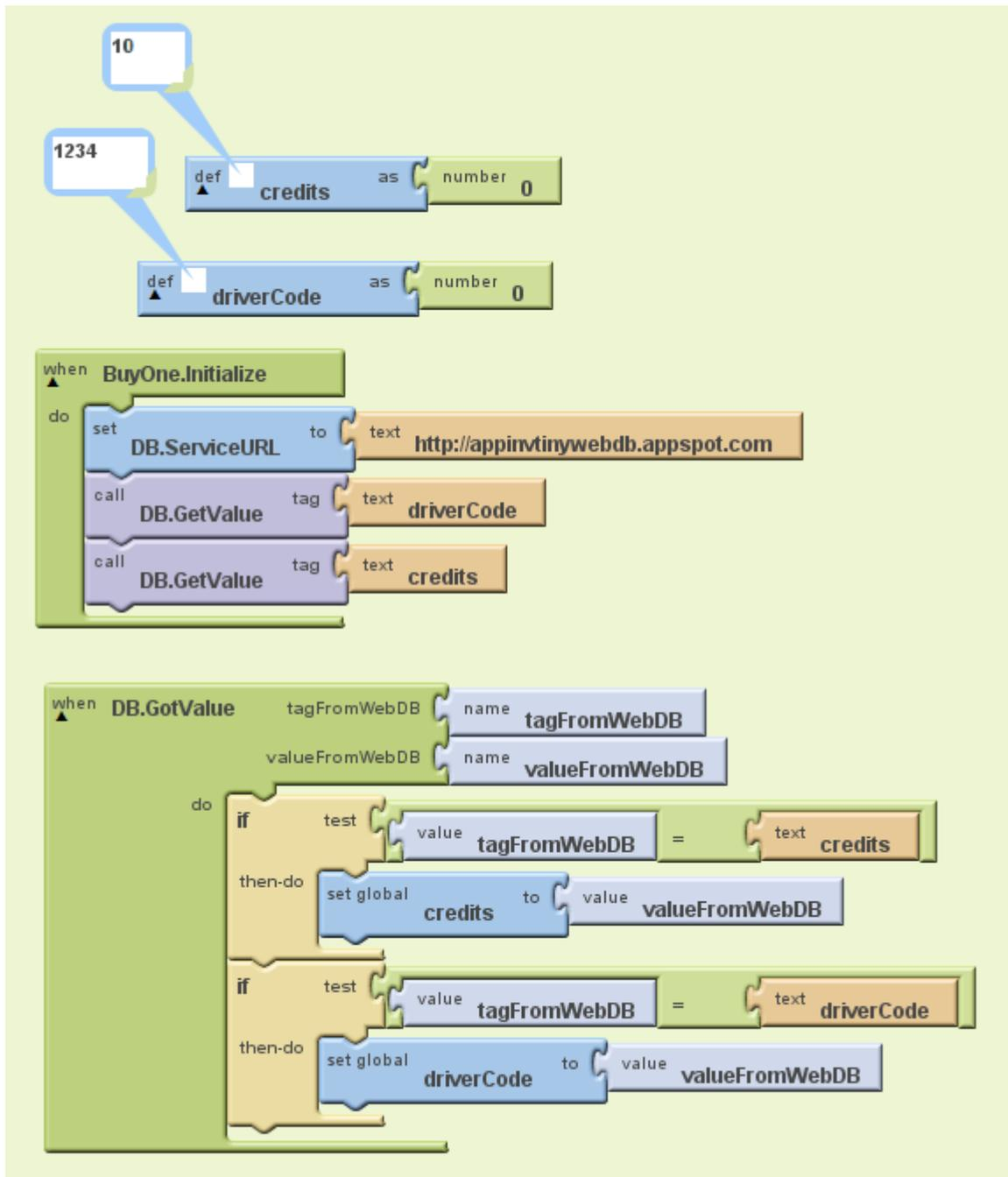
This is what happens when the buy ticket button is pressed. First of all the cost of the ticket is 3 or 5 depending on whether the return check box is ticked (by default it is not). Then the drivers code is checked to see if it is correct. If it is then the total number of credits – the cost is checked to see that it will be 0 or above and if all of that is correct then the details of the ticket are saved to the database.
