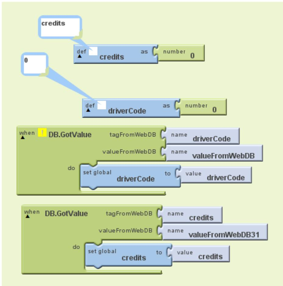
I hadn't realised the correct way to get information from this web database; this is the final version that works out what the 'tag' from the web is and puts it into the correct value.
